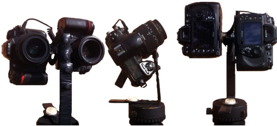
Figure 7. Manual Stereo Panoramic Mount with pair of Nikon DSLR cameras. The mount keeps the cameras rotating vertically through the lenses entrance pupil, and keeps the horizontal rotation of the lenses as close to the entrance pupil as possible. This mount allows the photographer to capture a full 360x180 degree image.
