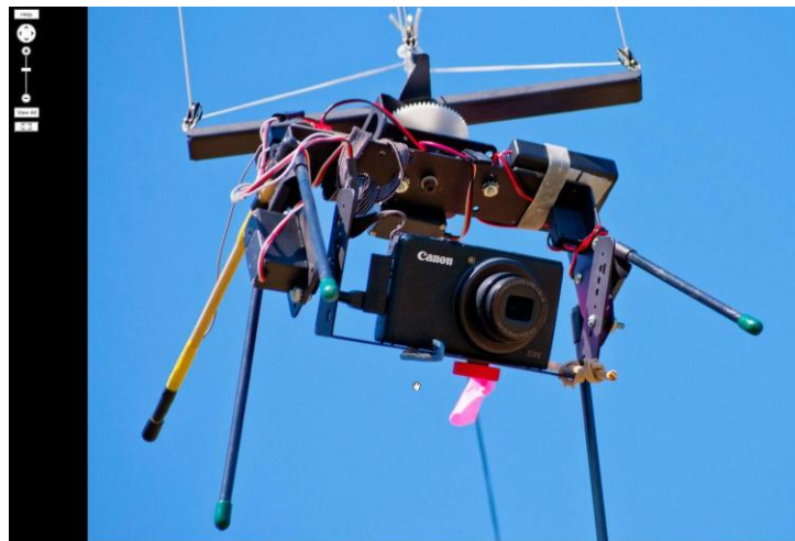
Figure 6. A single camera is kite suspended from a motorized mount by Chris Fastie. [7]
