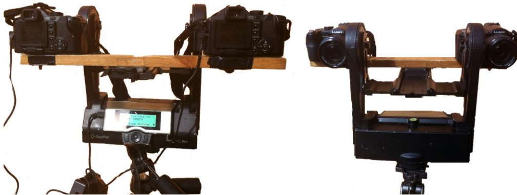
Figure 8. GigaPan Robotic Panoramic Mount with a pair of Panasonic FZ50 digicams mounted on a horizontal board. The camera separation allows for the hyperstereo capture of distant scenes, but the distance between the lenses would preclude image stitching success with subjects that are close to the cameras due to parallax error.
